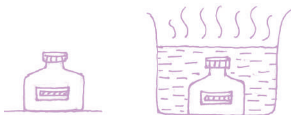
Fig. 14.9 Loosening a metal cap by heating it
