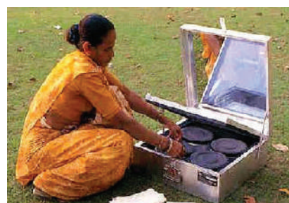
Fig. 12.4 Box type solar cookers
